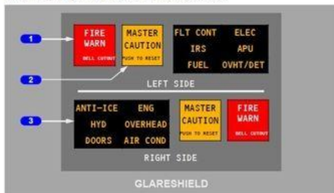
Fire Warning and Master Caution System
